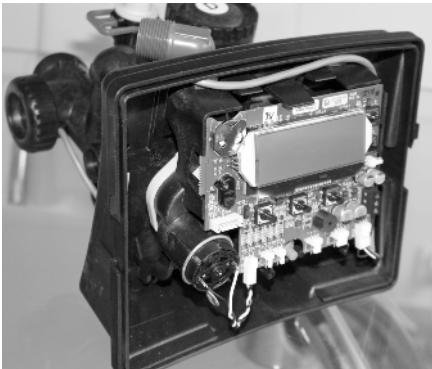
Step 2: Raise the ratchets with special attention (see photo). Pull out the element on which the controller is installed by pushing it gently.
