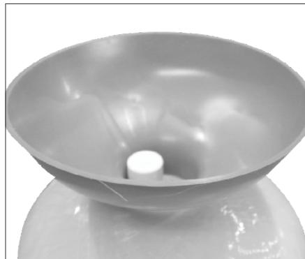
Step 4. Fill in the cylinder with the proper bed.
